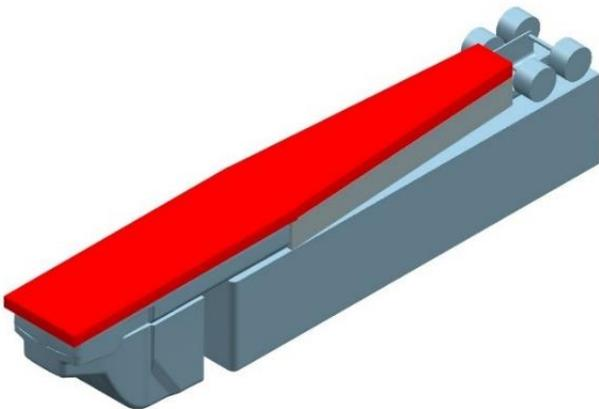
**Figure 2:** a) GCM with device configuration #12 (Ramp 6° - Side Skirt 4°) and b) the channel location highlighted in red
