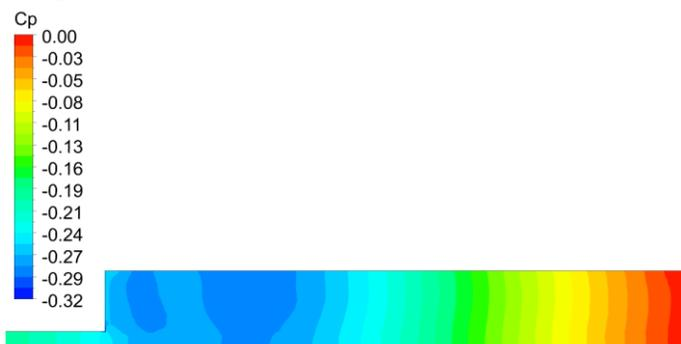
**Figure 5:** Pressure contour at the centerline of the baseline configuration
