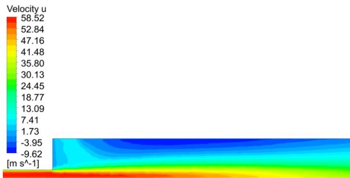
**Figure 4:** Velocity contour at the centerline of the baseline configuration
