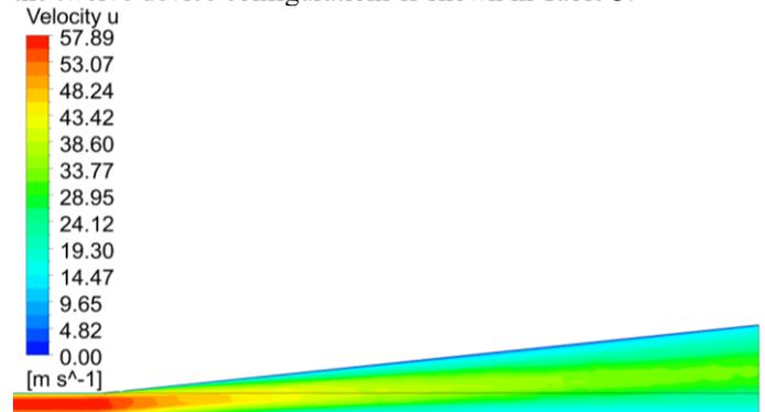
**Figure 7:** Velocity contour at the centerline of device configuration #12 (Ramp 6° - Side Skirt 4°)
