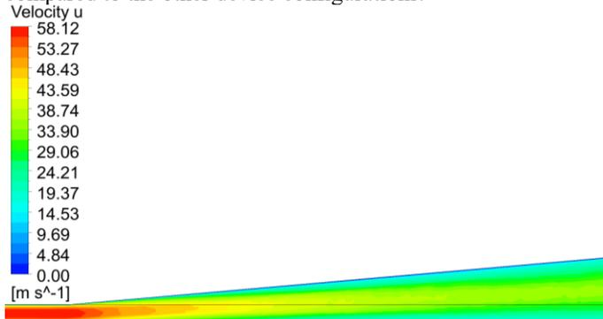
**Figure 6:** Velocity contour at the centerline of device configuration #9 (Ramp 5° - Side Skirt 4°)
