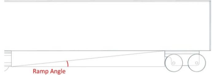
**FIGURE 1:** a) Proposed underbody drag reduction device attached on the underbody of the GCM b) Bottom view of the device indicating the side skirt angle c) Side view of the device indicating the ramp angle
