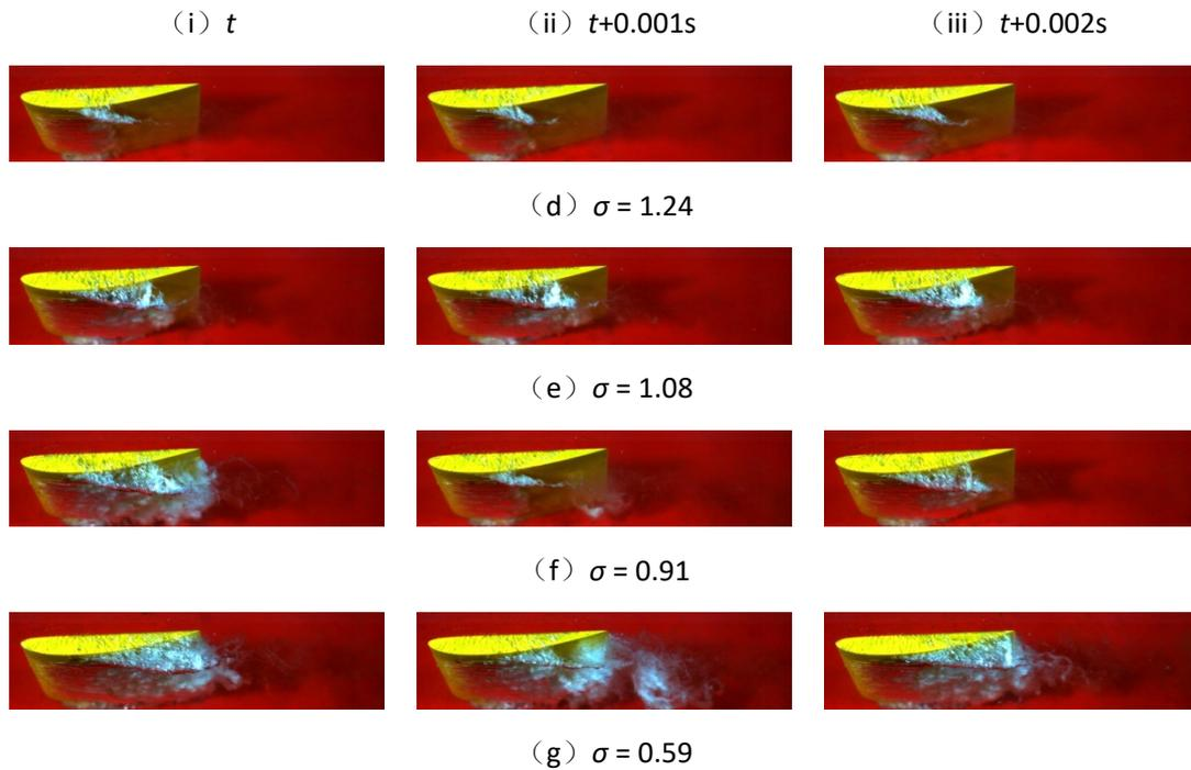
**Figure 4** Flow patterns of cavitation around the hydrofoil with different cavitation numbers
