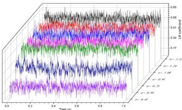
**Figure 5** Time evolution of the vibration with various cavitation numbers
