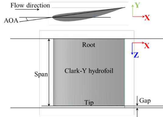
**Figure 2** Schematic of the rectangular Clark-Y hydrofoil with tip clearance
