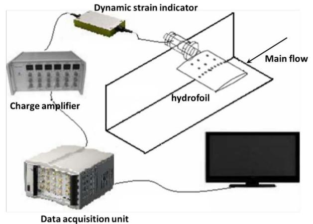
**Figure 3** Hydrofoil vibration measurement system
