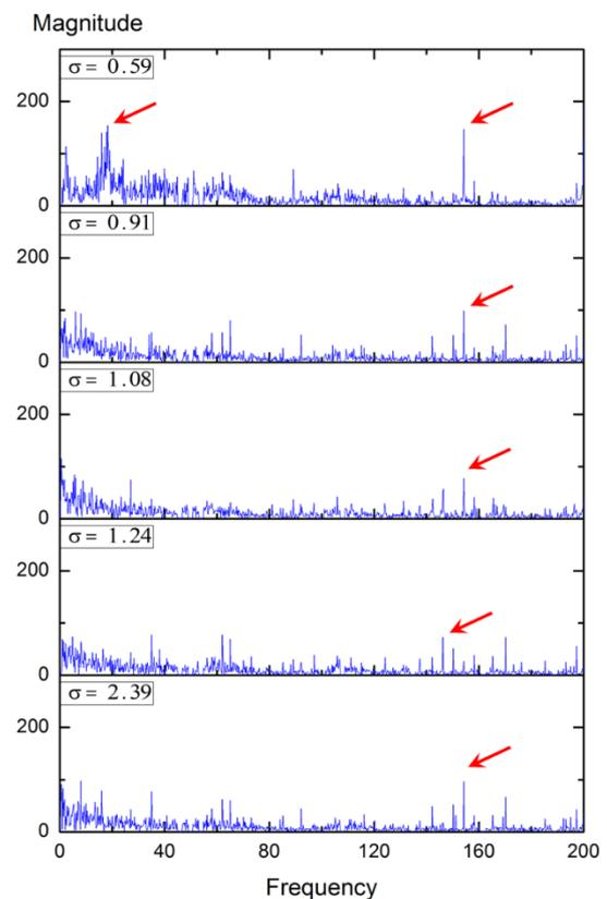
**Figure 6** The frequency spectrum of hydrofoil lift with different cavitation numbers
