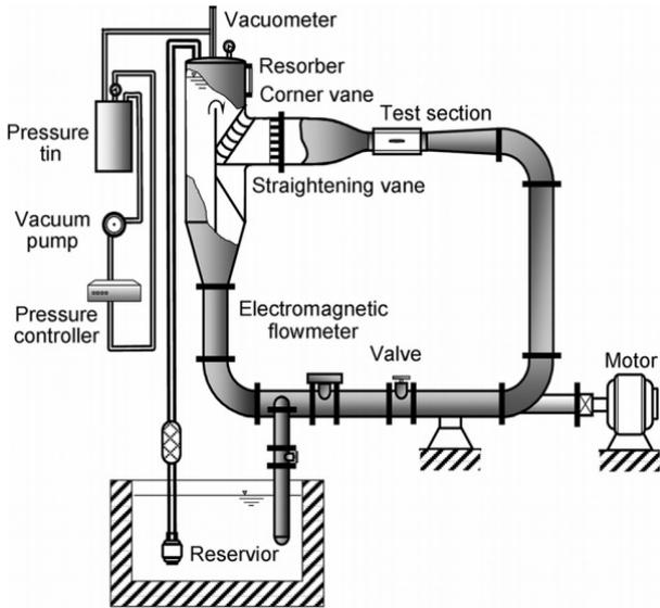
**Figure 1** Schematic of the cavitation tunnel
