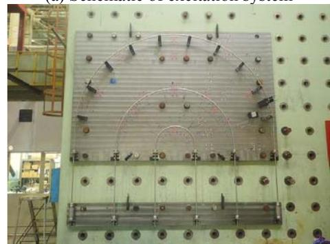
(b) U-tube used for excitation test
