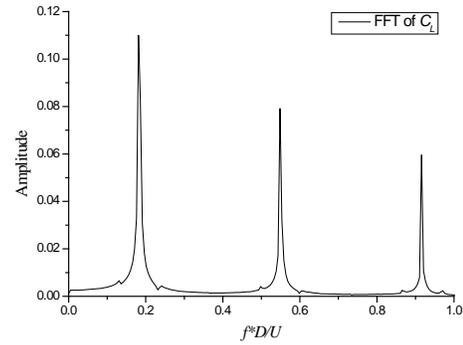
**FIGURE 12:** FFT FOR  $C_L$  IN CAVITATING FLOW
