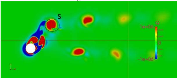
**FIGURE 4:** VORTEX MODE IN NON-CAVITATING FLOW WHEN  $F^*=0.9$  (THE VORTEX STRUCTURE IS REPRESENTED BY THE Q-CRITERION [21])
