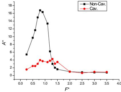
**FIGURE 8:** THE DIMENSIONLESS OSCILLATING AMPLITUDE  $A^*$  UNDER DIFFERENT  $F^*$ .
