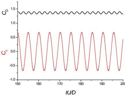
**FIGURE 9:** LIFT COEFFICIENT AND DRAG COEFFICIENT ON THE STILL CYLINDER IN NON-CAVITATING FLOW.
