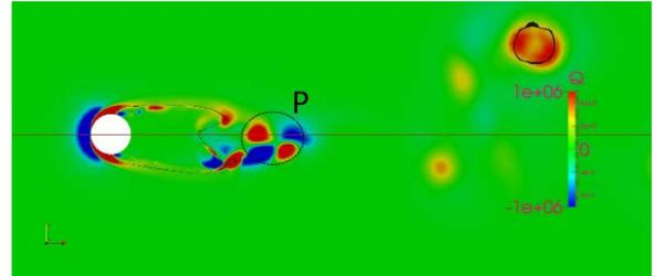
**FIGURE 7:** VORTEX MODE IN CAVITATING FLOW WHEN  $F^*=0.7$
