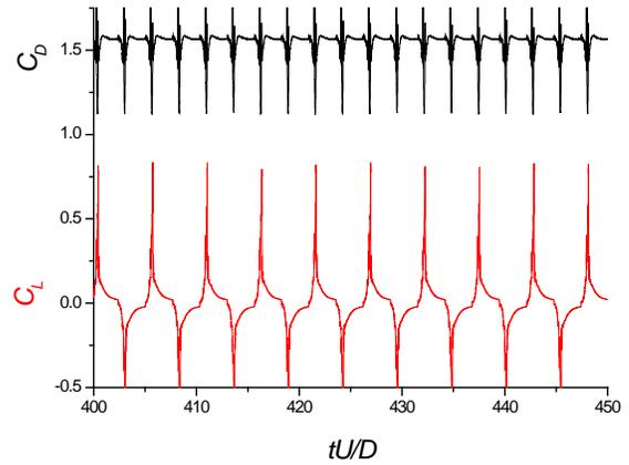
**FIGURE 11:** LIFT COEFFICIENT AND DRAG COEFFICIENT ON THE STILL CYLINDER IN CAVITATING FLOW.
