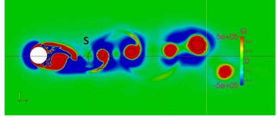
**FIGURE 5:** VORTEX MODE IN CAVITATING FLOW WHEN  $F^*=0.9$  (THE BLACK LINE ARE THE ISOLINE OF  $\alpha =0.9$ )
