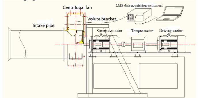
**FIGURE 3:** The centrifugal fan vibration decoupling test platform
