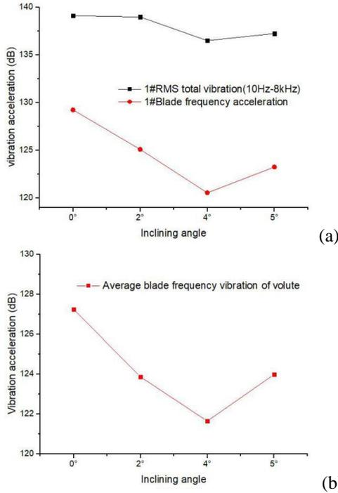
FIGURE 7: The vibration variation curve of tongue area and the volute in different angles
