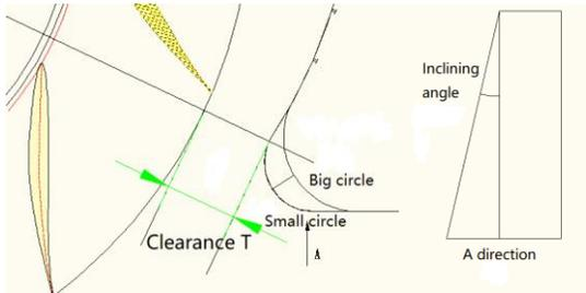
**FIGURE 1:** Volute tongue clearance and inclining angle
