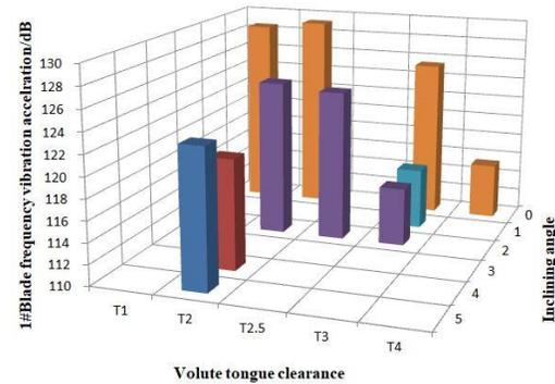
(a) Blade frequency acceleration of point 1#
