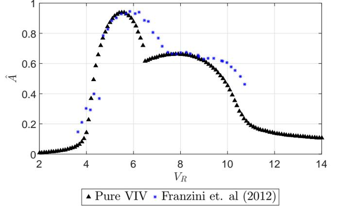
**FIGURE 2: PURE VIV SIMULATION AND EXPERIMENTAL DATA.**
